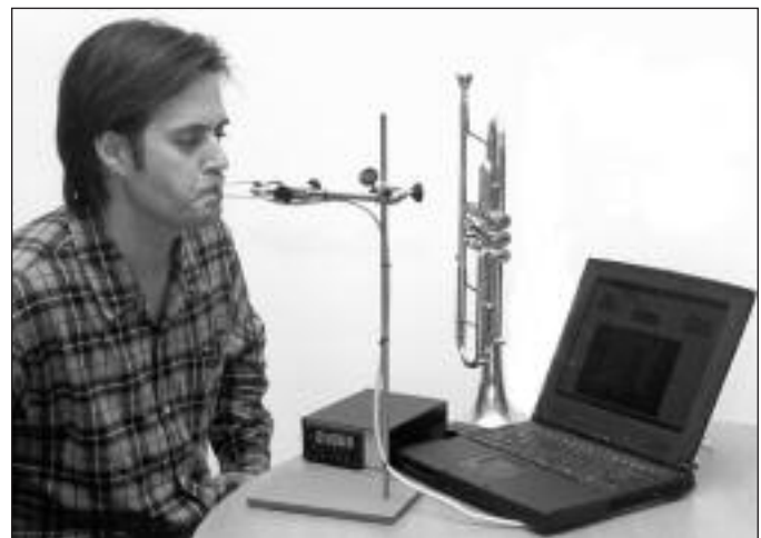
Figure 5: TEDEL4, a system to measure force and resistance of orbicularis oris muscle
